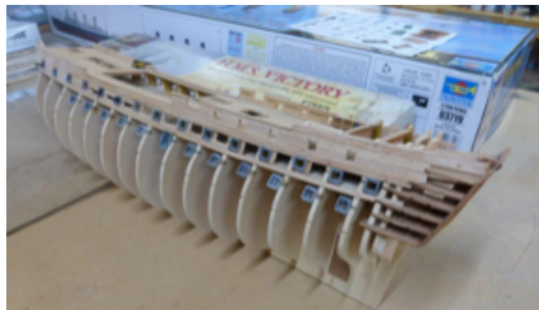
Port quarter looking forward. Note that the gunports are fixed prior to planking.
