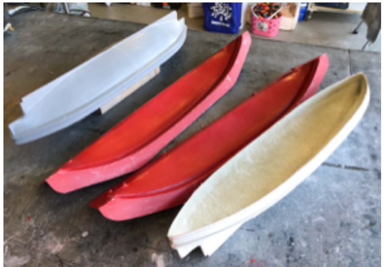
The 3d printed hull, the fiberglass mould and the fiberglass hull.
