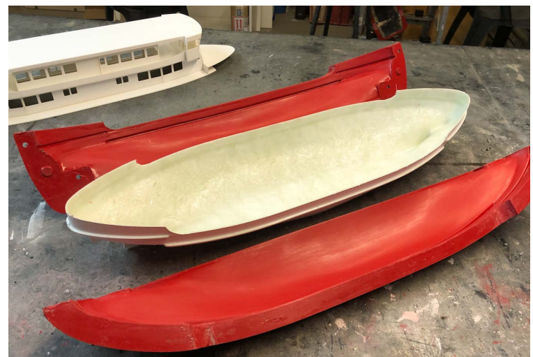
The fiberglass mould and a hull with a styrene superstructure
