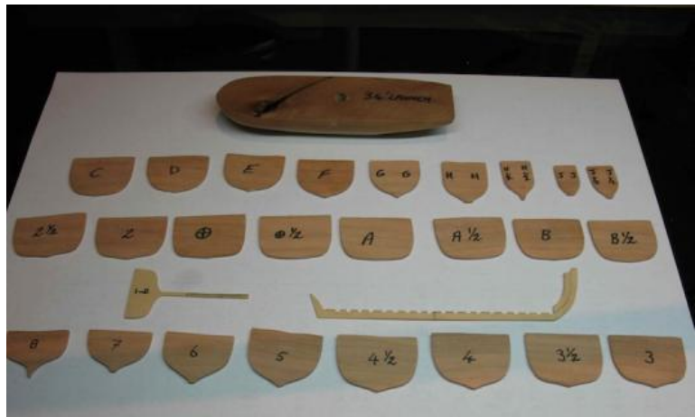
The next step was to add a single strip of 1/32" boxwood to the keel and then mark and notch it for the frames, using the building board notches as a guide. Below.
