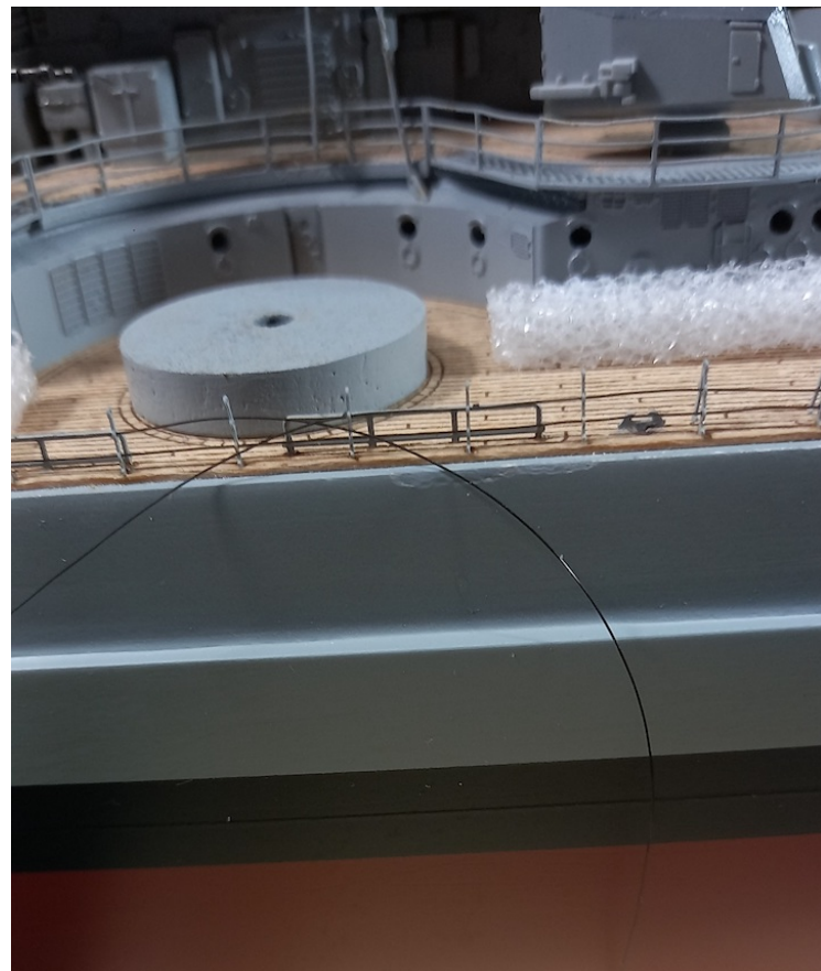
Start of threading the main deck railings to over 200 stanchions - the beginning of the end.
