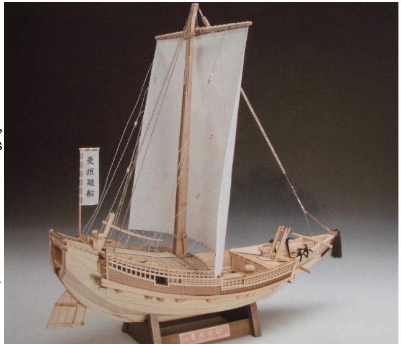
Higaki Kaisen model, very similar to Kitamaebune, but with full internal structure
