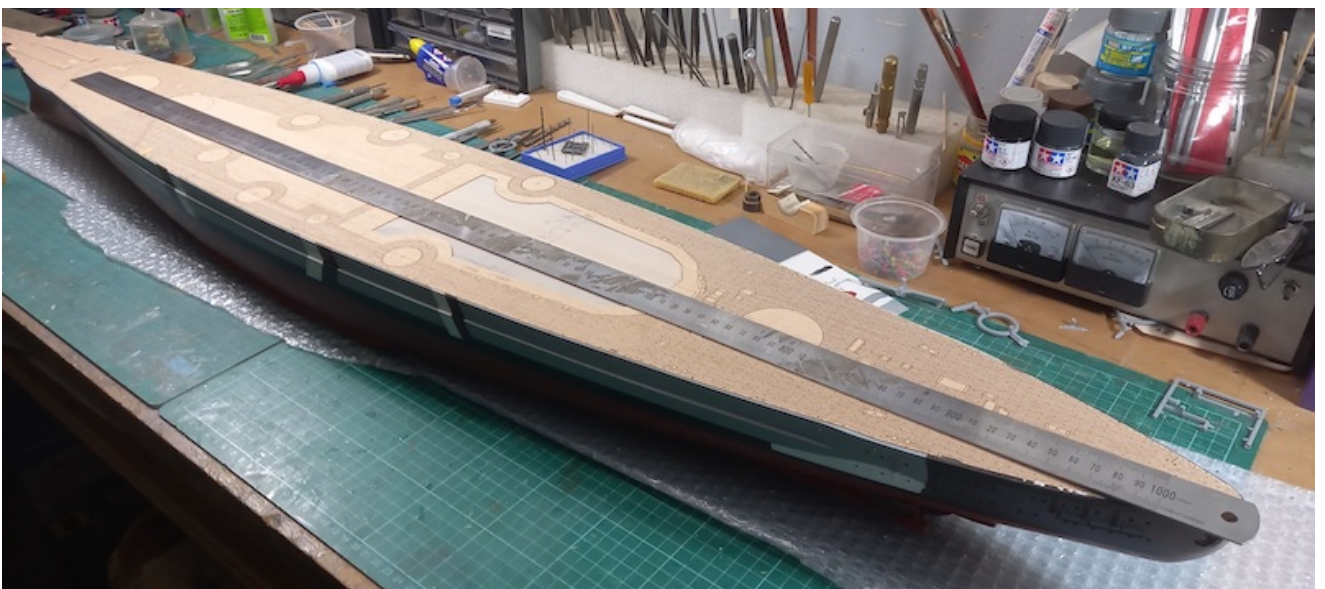
Above - Deck sections being glued on hull. Below - Checking alignment of deck sheets.
