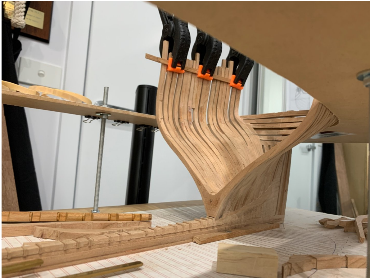
Figure 10 - The first two full frames installed
