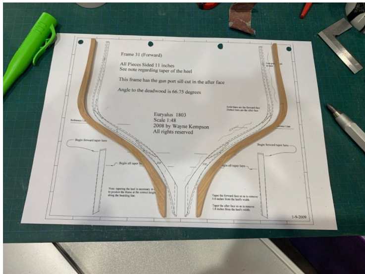
Figure 2 - Cant Frame assembled and checked against template
