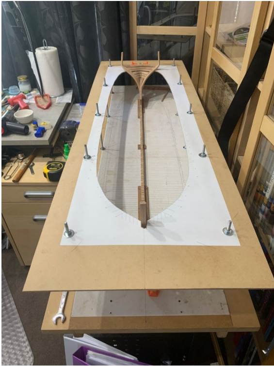
Figure 6 - Reference Board in place
