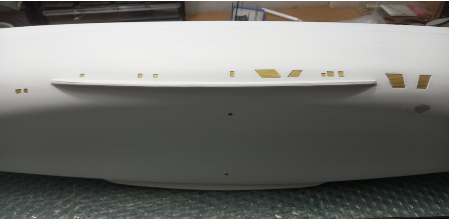
Above - Inlet gratings installed
