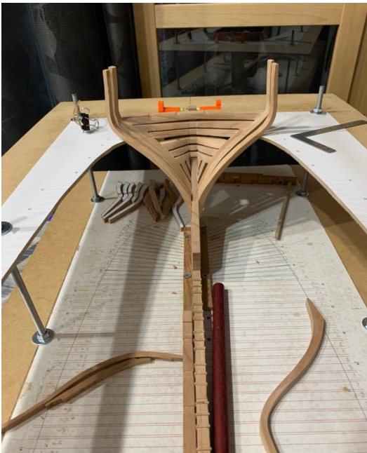
Figure 7 - First Cant Frame 31a glued in.
