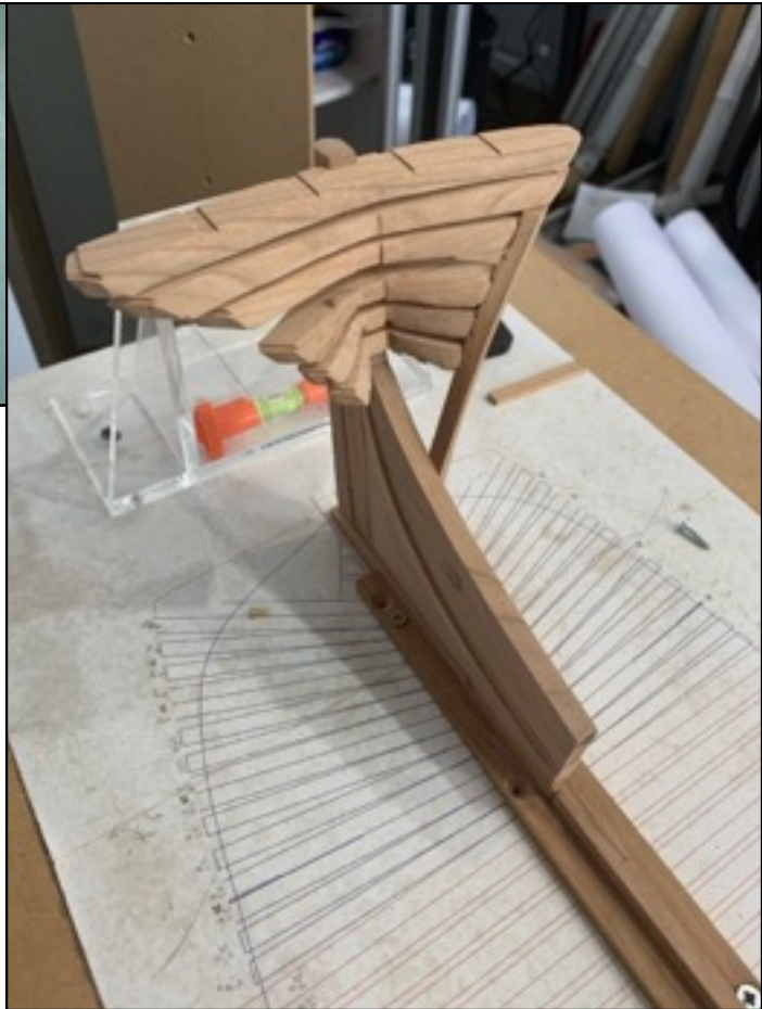
The photo shows the stern assembly on the keel, It also shows the first of Russell's original components being fitted to the rebuilt model; the port half-fashion piece fixed to the ends of the transoms.
