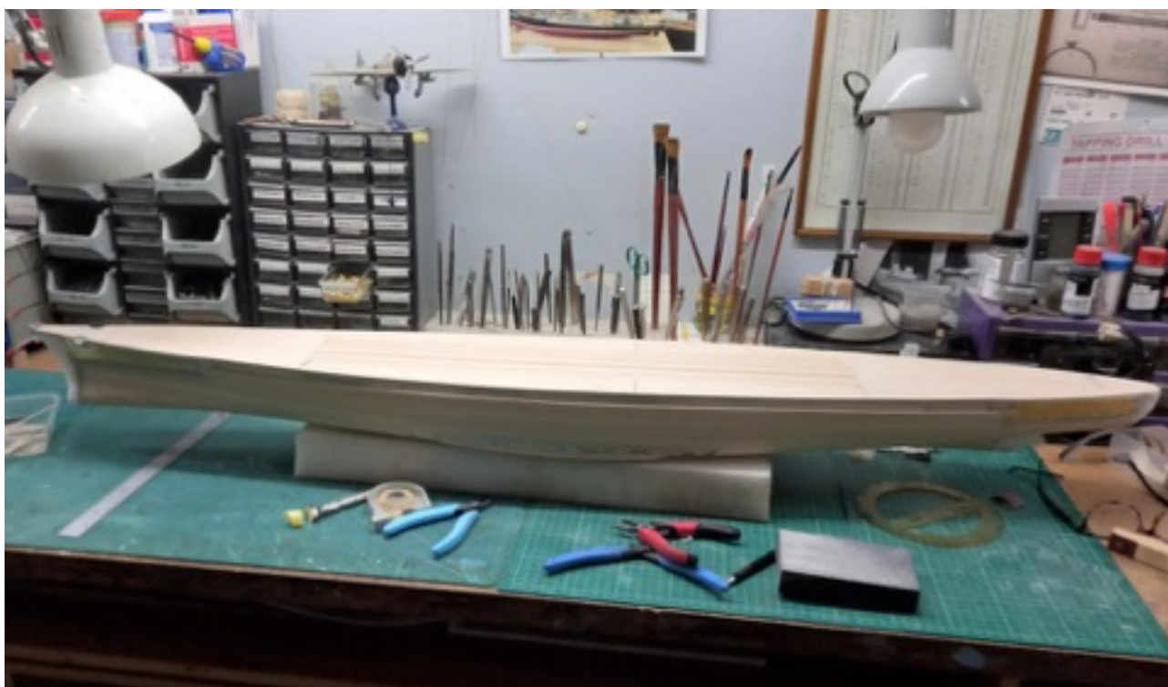
Hull planking completed, ready for top coat and fittings.
