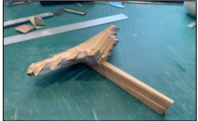
Stern post and transoms dry fitted.
