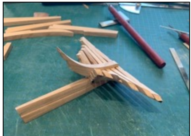
Sternson knee dry fitted to the stern assembly
