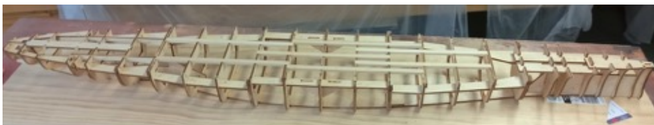
Above - All the frames installed and below - completed framing.
