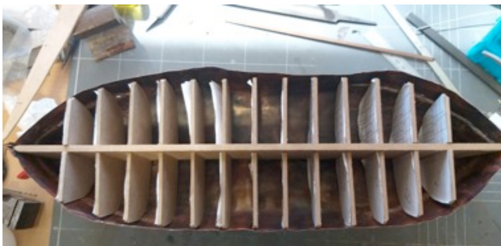
The internal cross sections have the top edge notched to allow the fitting of the internal gunwale and are sufficiently "loose" to allow the central internal "keel" to be removed and the formers rotated to be removed with the gunwale in permanent position. This framework will also allow adjustments to the hull sections when soldering the stem and stern to the keel.
