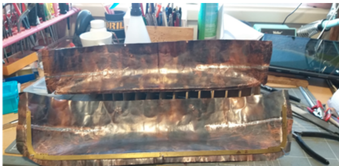
The two formed hull sections with one initially bolted to the keel. The hull sections above have not yet been trimmed to the final size.
