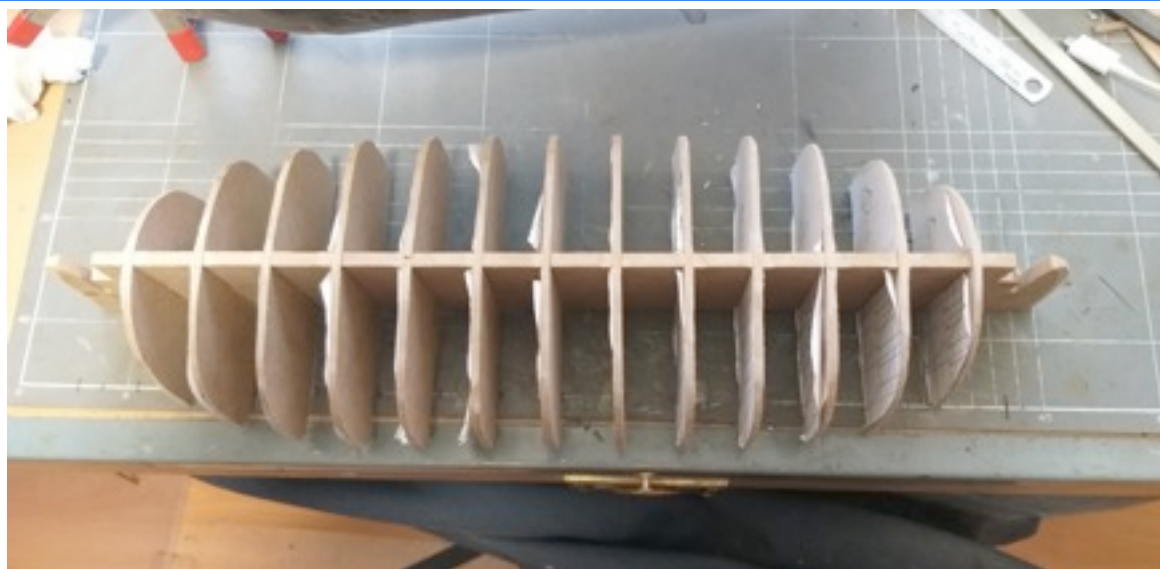
The internal cross sections have the top edge notched to allow the fitting of the internal gunwale and are sufficiently "loose" to allow the central internal "keel" to be removed and the formers rotated to be removed with the gunwale in permanent position. This framework will also allow adjustments to the hull sections when soldering the stem and stern to the keel.
