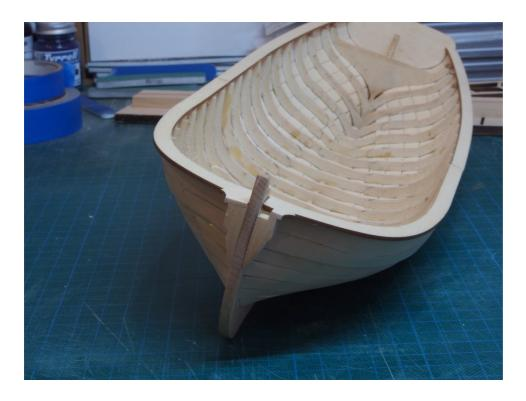
With the bolsters in place, I was then able to go ahead and thin the cap rails. I used a scrap of 1/32" material to guide the formation of the outboard edge to a uniform overhang, then using a pair of compasses marked a line 5/32" from the outboard edge to guide the thinning of the inboard side.
