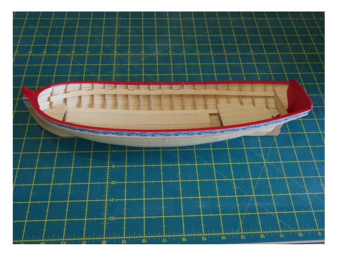
The thwarts have been built and fitted to the model, though not glued in yet. The cockpit seats have also been built, fitted and glued in place. I added small tabs to the underside of the aft thwart and the aft end of the cockpit seats to provide additional landing places to help keep everything aligned. More work to do on the thwarts, and lots of painting in the cockpit...
