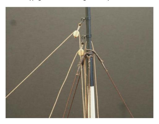
I seized the deadeyes into the ends of shrouds prior to installing the shrouds and seizing them to the mast. I decided to add a throat lashing to the deadeyes and it turned out quite well. To complete the lanyards, I threaded the ends between the throat lashing and the upper deadeye and then tied a couple of half hitches. As these were working lines, I thought it would be unrealistic to seize these to the shrouds, even if it would have looked neater!
