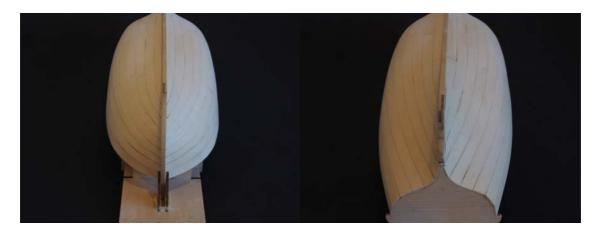
The whales were then added. I did these in reverse order, working down from the gunwhale in order to correct any minor misalignment at the bow. I used a sharp chisel to pare down the forward end as it approached the rabbet. The aft end was simply sanded thinner for the last half inch or so. All of the holes have been drilled in preparation for the monofilament "nails".
