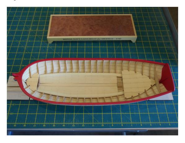
I have completed preparing and installing the risers. Using the heat/hair-dryer method to pre-bend the risers makes attaching them much easier. I picked up a tip from a couple of other logs about using a small T-square jig to position the risers at the correct height at each frame.
