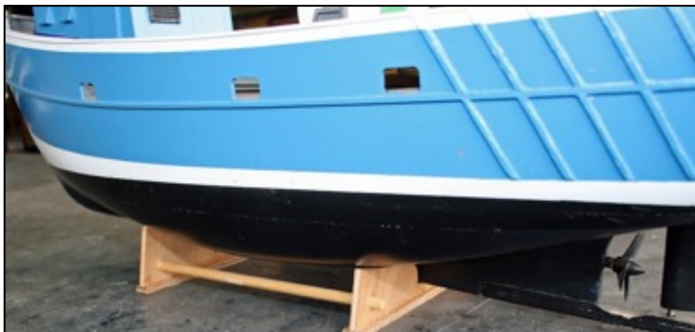
An example of an ineffective stand. Made from very light material, nowhere near big enough to adequately support the model and the unfinished timber does not blend well with the colour of the model.
