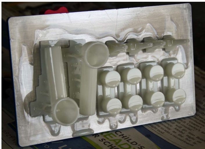
Parts straight off the printer, still attached to the build plate dripping excess resin.
