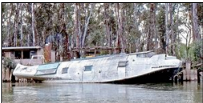
A Catalina hull prior to conversion to a houseboat (nose gun turret intact, but waist blisters removed), probably on the Murray River
