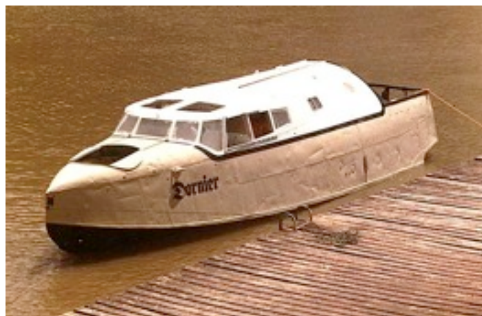
And a Dornier echo in Australia - this houseboat photographed on the River Murray was built around a Dornier fuselage.
