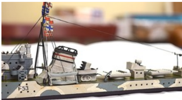
Port lifeboat, pinnacle and funnel stay. Ammunition lockers can be seen on the multiple machine gun platform.
