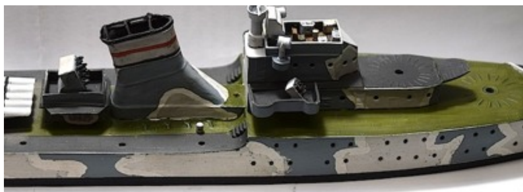
Open bridge showing fittings (crew added later), fire control, range finder and starboard and port searchlights. Multiple machine guns are sited on the bridge platform just below the searchlight. The winch at deck level to the right of the funnel was where one of the “additional” deck holes was located (see Funnel Area Section).
