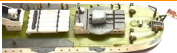
Rear deckhouse with 4.7" guns, winches, depth charge chute, depth charge hoists, jack staff and ensign.
