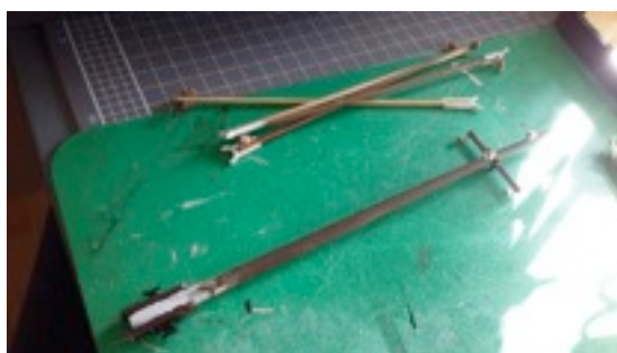
Figure 19 Completed and rigged Mast, Boom and Gaff
