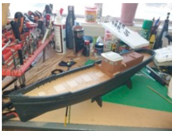
Figure 7 Superstructure, Breakwater and Side Platforms Installed
