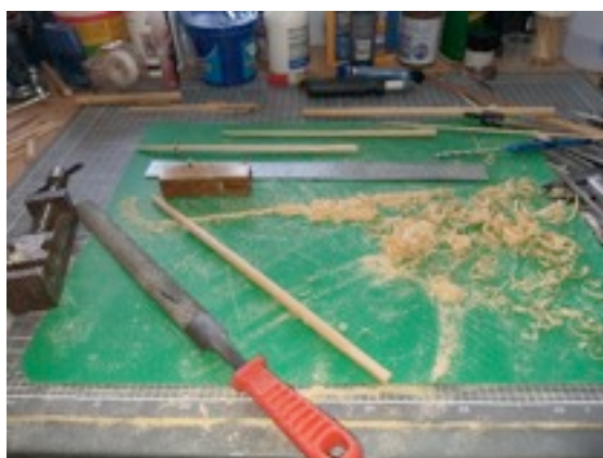
Figure 18 Mast, Boom and Gaff Tapering
