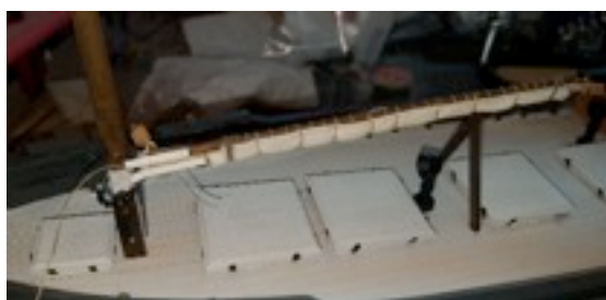
Figure 20 Boom, Gaff and Furled Sail Installed
