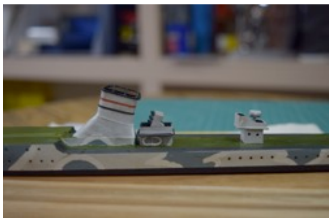
Fig 9: Funnel, pom pom gun, life rafts and searchlight deck.
