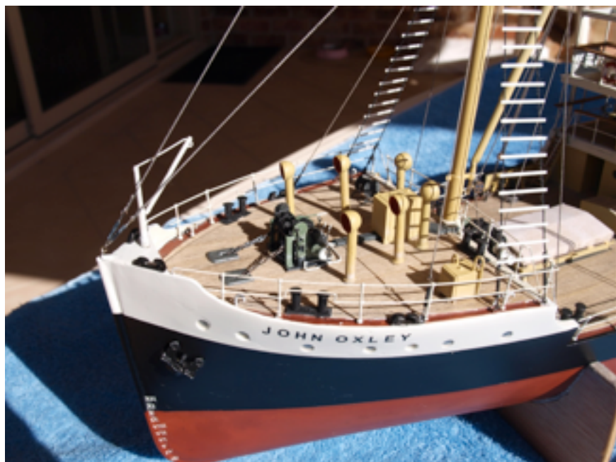
Well deck showing cargo winch also cargo hatch. The rails can be removed, bulwarks fixed in their place (see below). Below: bridge and boat-deck.
