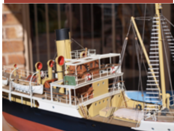
Well deck showing cargo winch also cargo hatch. The rails can be removed, bulwarks fixed in their place (see below). Below: bridge and boat-deck.
