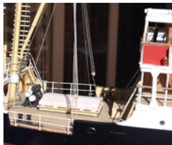
Well deck showing cargo winch also cargo hatch. The rails can be removed, bulwarks fixed in their place (see below). Below: bridge and boat-deck.
