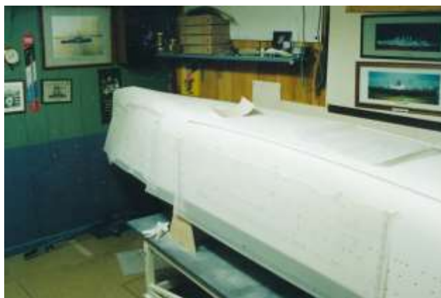
Hull repairs completed and waterlines being marked up. Below – Hull painting completed.
