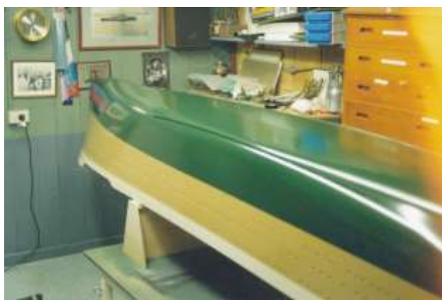
Hull repairs completed and waterlines being marked up. Below – Hull painting completed.
