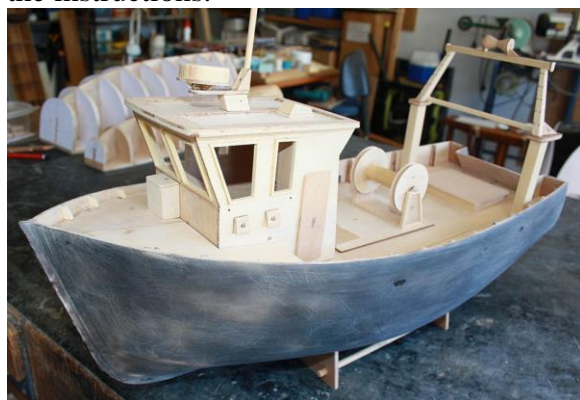
The major components of the model constructed. Note that the hull has been covered in fibreglass.
