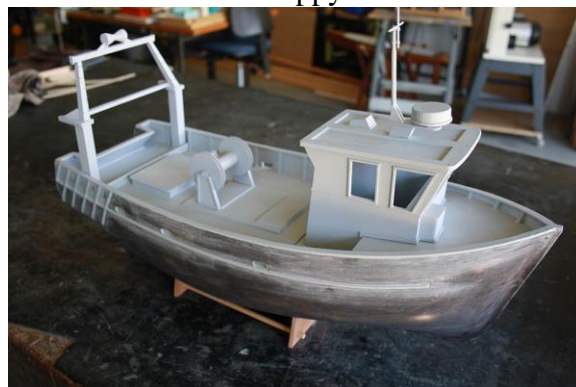
Several coats of paint were used to fill the grain of the wooden components.
