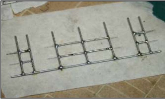
Railings 2 - Railings made using masking tape to hold parts still.
