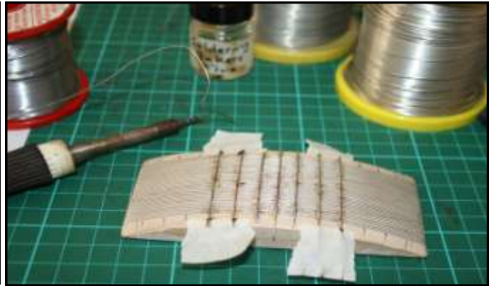
Radar 1 - The start of a radar being soldered together using double sided tape on a wooden former to get the correct shape.
