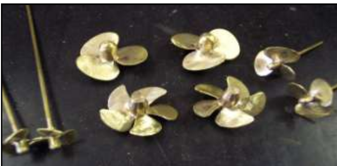
Propellers 1 – A selection of home made model ship propellers that have been soldered together.
