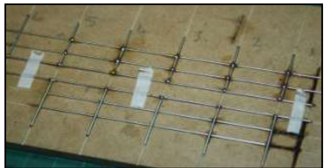
Railings 1 – Small pieces of tinned copper wire soldered together using a wooden jig to make railings for a model ship.
