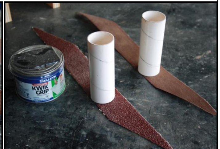
Abrasive belt cut to size and ready to be glued onto the PVC drums.
