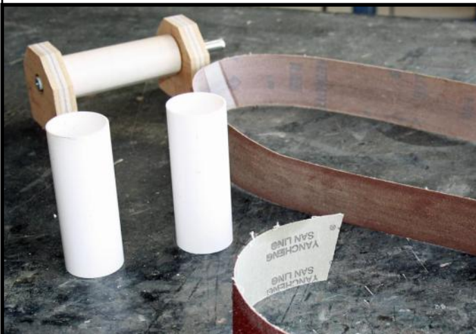
Sanding drums cut from PVC pipe and abrasive belts.
