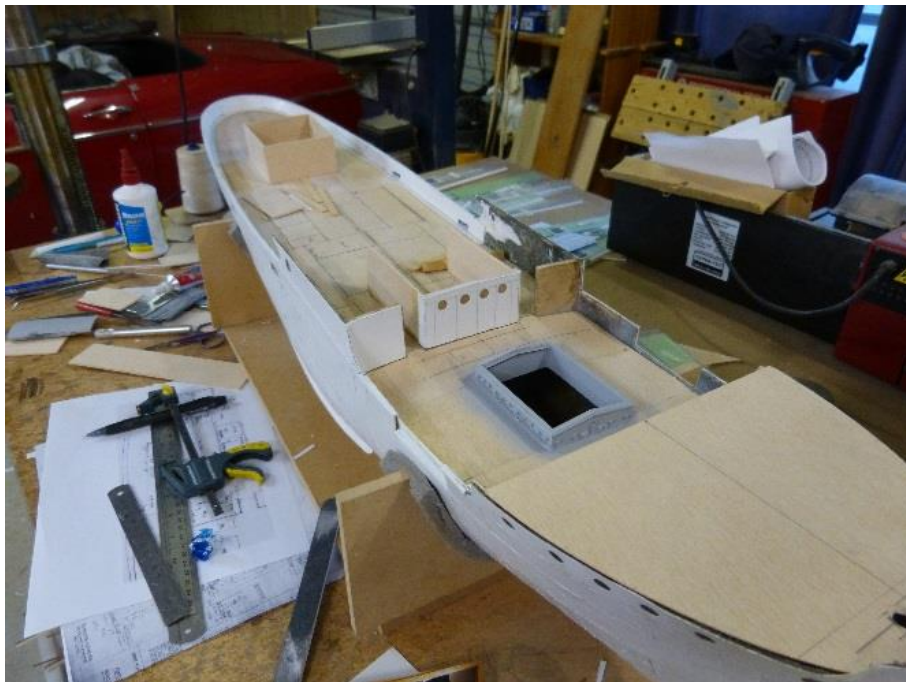
Main deck hatch and coaming completed. The accommodation aft is a little complex and is made up from a series of ply bulkheads, again lined with plastic card. All portholes are punched out, drilled where required and portholes inserted.
