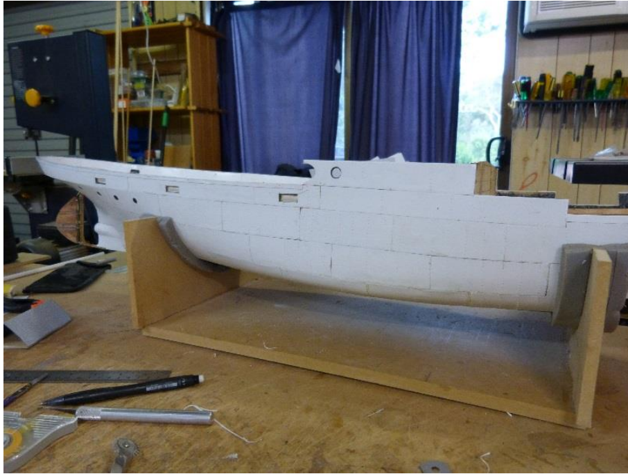
Hull plating is now completed, freeing ports added, stern frame fitted.
