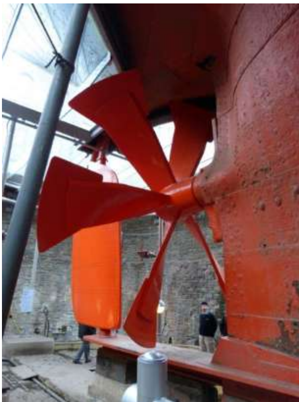
The reconstructed propeller. The balanced rudder, also new, is described in Photo 7
