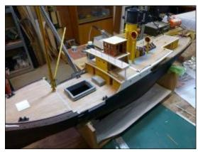
Above: General view. All the decks, with the exception of the wheelhouse top are fixed, as is the funnel and ventilators. The white square forward is the start of the forward windlass- a bit to do yet!
